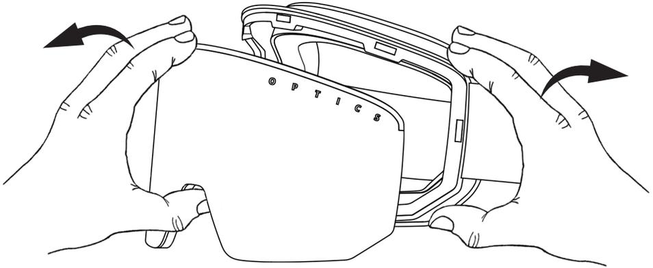
EN: To use a new lens place it on the frame and make sure that all magnets are aligned.
